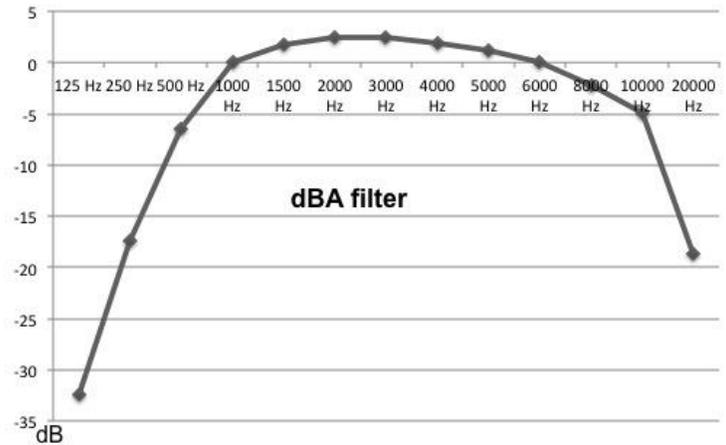
**Figure 2.** dBA filter used in the study (3BKAP software)
