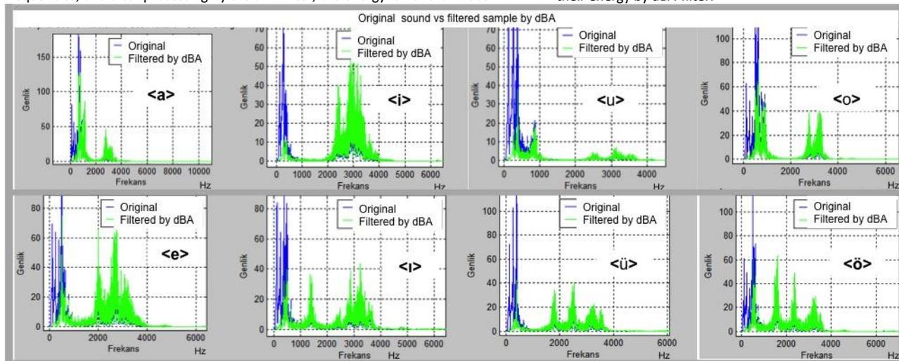
**Figure 3.** Effect of dBA filtering on the original files of the vowels is seen. Blue drawings pointed out the deleted energy by dBA filter; the green drawings are the rest of the speech sample of the vowels
